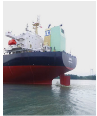
2. Scrubber retrofitted on M/V Xenia, 2006, Post-Panamax, DWT 87,000
